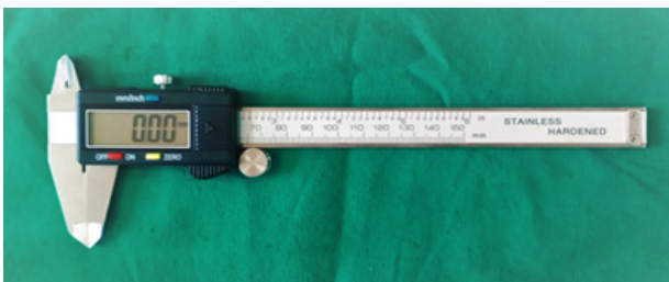
Figure 1) Photograph showing digital vernier caliper.
