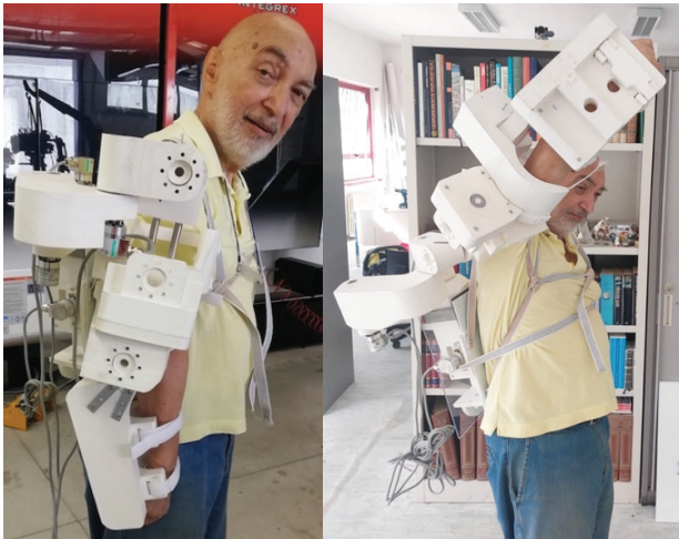
Figure 11) The initial images of the half exoskeleton provided valuable insights. Two important lessons were learned: firstly, the straps must be very tense, and secondly, the first strap on the forearm must be positioned very close to the elbow. Additionally, it was observed that the position of the fourth encoder must be above the third bar that holds the motor on the shoulder. In both cases, the hinge that should bear the motor is aligned with the clavicle. These observations highlight the importance of precise adjustments and alignments for optimal functionality.
